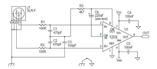
In practise, we only added some power supply related components to this by THAT recommended circuit. Even though the IC has transient voltage suppressor diodes on board, we added better (TVS) ones.
