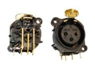
The second one we provide with an XLR female chassis connector. You can decide whether the connector body is connected to Signal- or power ground or not at all, depending on your design. It can prevent hum either way.
